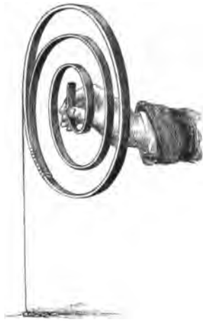
Action of a Watch Main-spring Illustration.
